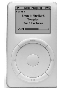
Figure 11.7 Apple's original iPod was controlled by four buttons, and a mechanical control wheel turned to move through menus and song lists. It held up to three thousand songs on a miniature hard disk drive with more than a thousand times the capacity of IBM's original RAMAC unit. Image created by Wikimedia user Miquel750-5303, used under the Creative Commons Attribution-Share Alike 4.0 International license.
