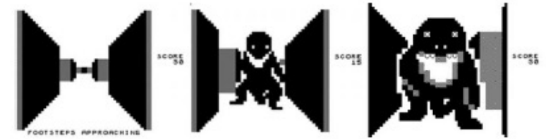
Figure 7.12 The programmers of home computers displayed great creativity. The ZX81 had a text-based display with special characters to represent block shapes and shading. 3D Monster Maze , programmed by Malcolm Evans in 1982, was a 3D maze, home to a rampaging Tyrannosaurus rex.
